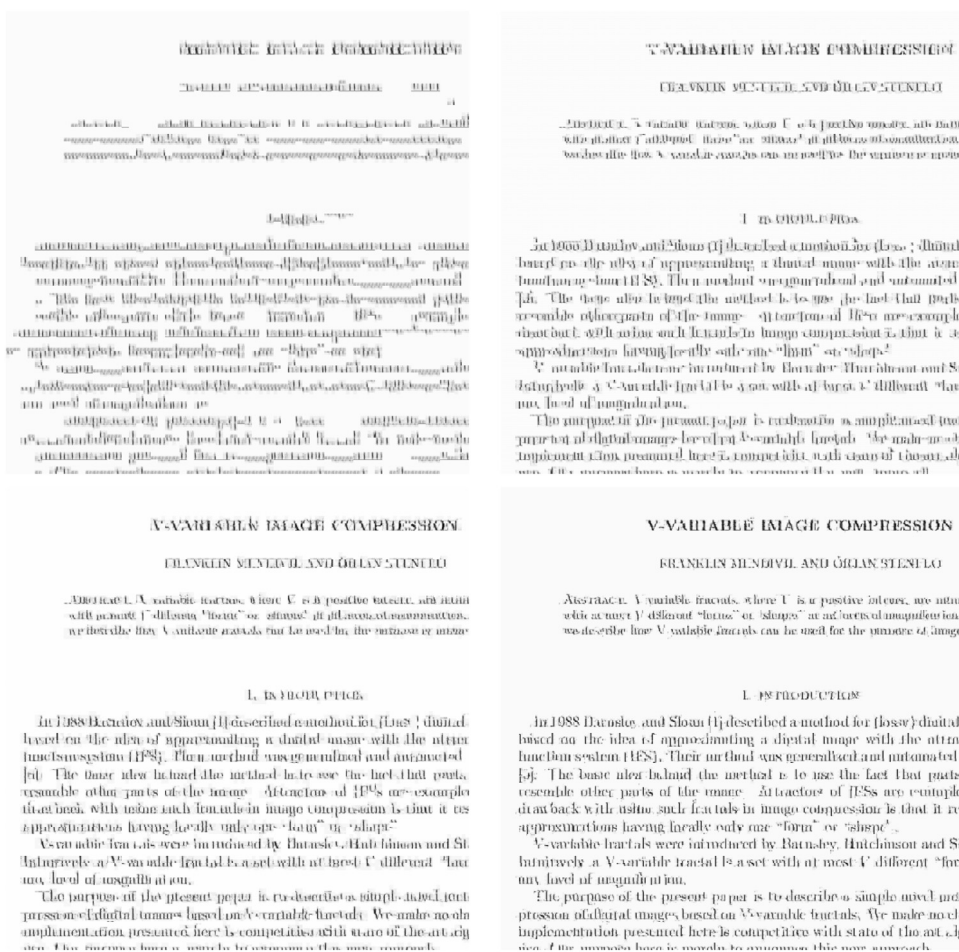
Fig. 6. V-variable approximations of Image2 with storage of size 1500 B (PSNR 16.7), 3000 B (PSNR 18.3), 4500 B (PSNR 19.4), 6000 B (PSNR 20.4).
