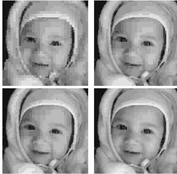
Fig. 5. V-variable approximations of Image1 with storage of size 1000 B (PSNR 24.0), 1500 B (PSNR 25.5), 2000 B (PSNR 26.1), and 2500 B (PSNR 26.7).
