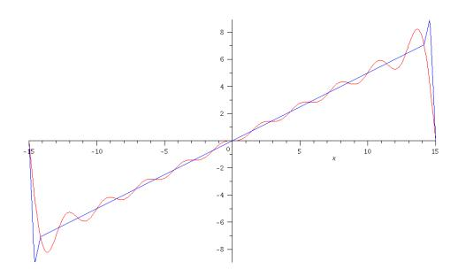
FIGURE 2. A piecewise linear shock and its Fourier approximation with 10 modes.
