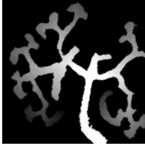
Figure 8.9: Geodesic distance function from the anchorage point (negative view of the supremum of the sections)
