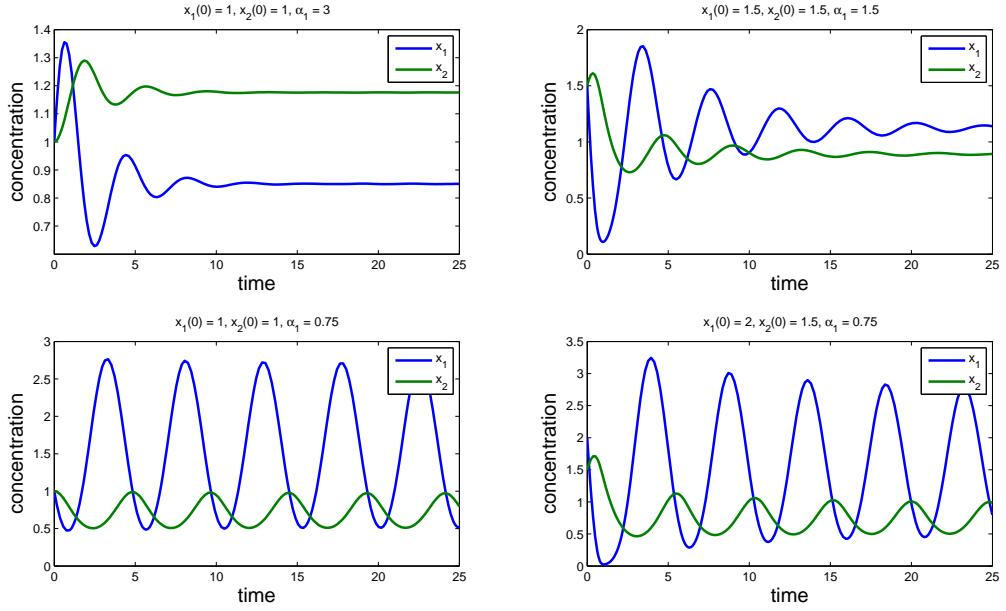
Figure 1: Different behaviours of the 2-dimensional system (Eq.(1-4)) depending on the initial concentrations and  $\alpha_1$ .
